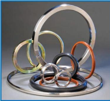
Ring Joint Gaskets are precision machined metallic sealing rings, suitable for high temperature and high pressure applications. By applying pressure to the seal interface through bolt force, the softer metal of the gasket flows into the micro-fine structure of the harder flange material, creating a very tight and efficient seal. They are available in several common profiles to suit a variety of industry standard flanges.
